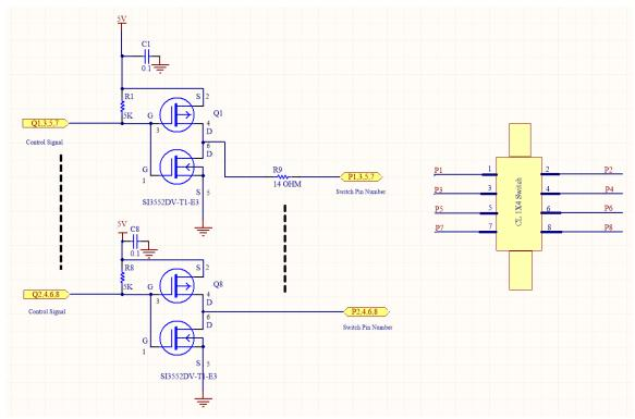
Usually, a clean power supply source will be sufficient. However, decoupling capacitors for the transistor supply rail are recommended depending on different applications. Minimum the current loop on the switching circuits will minimize the switching noise. For other layout recommendations, please refer to books or application notes from the IC manufacturer.
